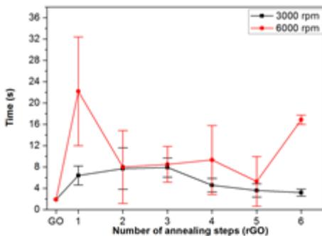
Figure 4: Comparison of response time to humidity for GO and rGO spin-coated at 3000 and 6000 rpm as a function of the annealing steps.
