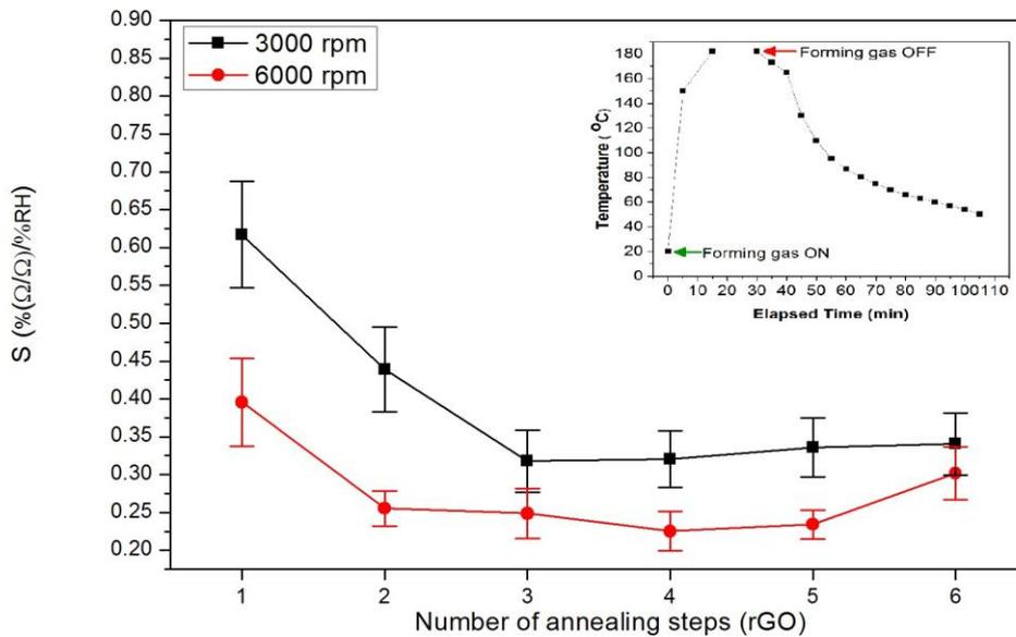
Figure 3: Sensitivity  $((R_{air}-R_{vac})/R_{vac}/\%RH)$  comparison of 3000 and 6000 rpm for six annealing steps and schematic of annealing process.
