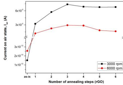
Figure 2: The effect of thermal annealing and spin speed of GO film on sensor's current (for  $V=7\text{ V}$ ) on air state.
