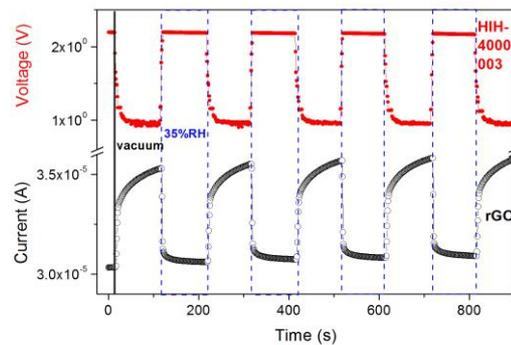
Figure 5: Response comparison of rGO sensor (3000 rpm, annealed steps:6) to commercial humidity sensor HIH4000 for 30% RH.
