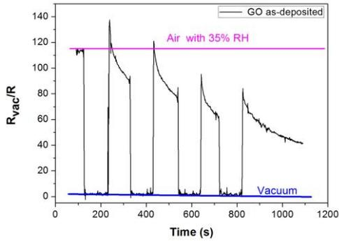
Figure 1: Response of spin-coated GO sensor to humidity (spin speed: 6000 rpm).
